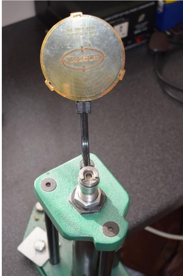
Priming tool that fit on top of a single stage press
