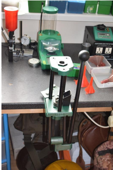
A single stage press mounted on a sturdy bench
