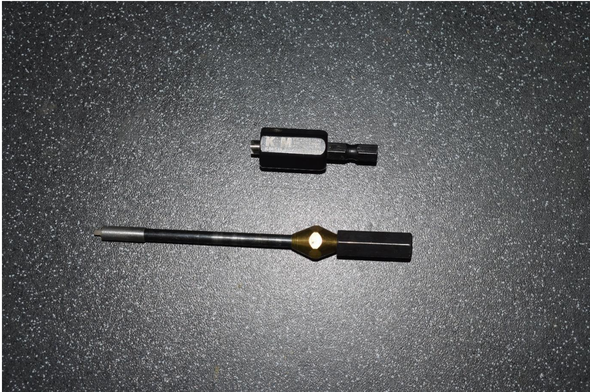
Top is a primer pocket uniform tool below is a flash hole uniform tool both can be fitted to an electric drill
