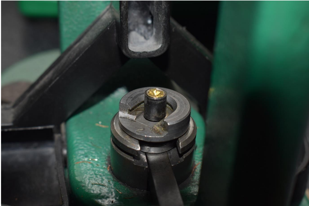
Primer mechanism fitted to the single stage press
