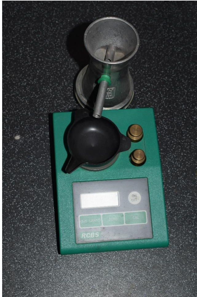
Powder trickle above an electronic scale
