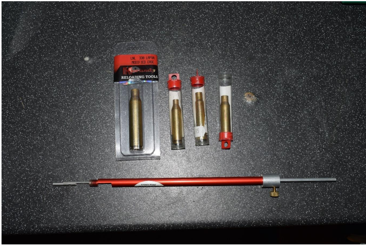
Bullet seating tool with modified cases this tool is used to work out the optimum bullet seating depth for a given bullet shape. Its for use in single loading not magazine fed rifles
