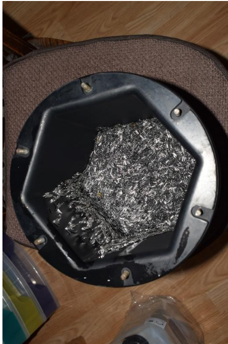
Steel pins in the wet tumbler
