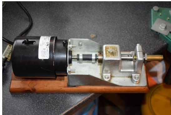
Electric case trimmer with de burring tool
